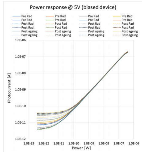
**Figure 9:** power response of a reference device biased during gamma irradiation up to 47krad(Si); in the range of interest, minimal variations were recorded i.e. lower than 2%
