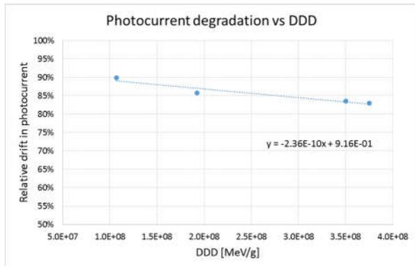
**Figure 12:** photocurrent degradation as a function of the DDD
