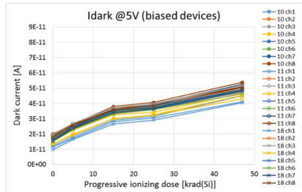
**Figure 8:** dark current degradation as a function of ionizing dose, on devices biased during radiation
