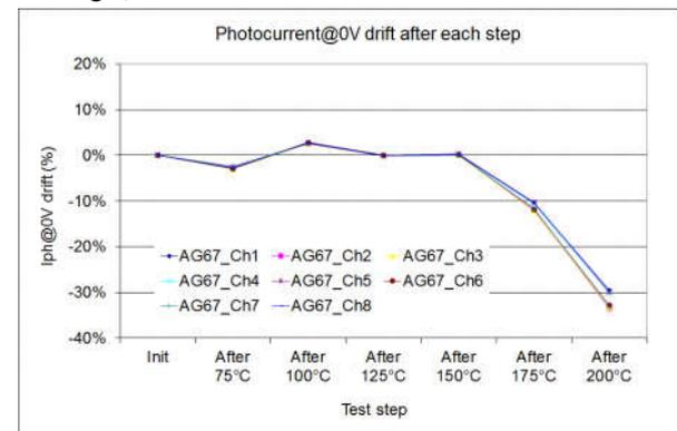
**Figure 3:** degradation in photocurrent during temperature step-stress
