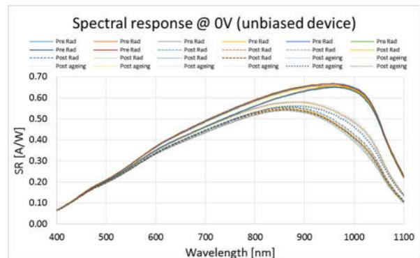
**Figure 10:** spectral response of one device unbiased during 60MeV-5.5E10p/cm<sup>2</sup> proton irradiation; comparison pre vs. post irradiation (degradation lower than -14%), and after ageing (lower than -12%)
