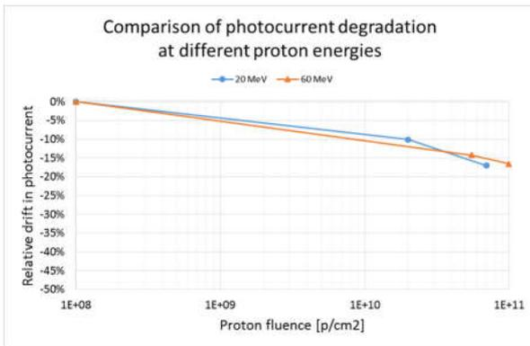
**Figure 11:** comparison of photocurrent degradation at 20 MeV and 60 MeV (averaged channels)
