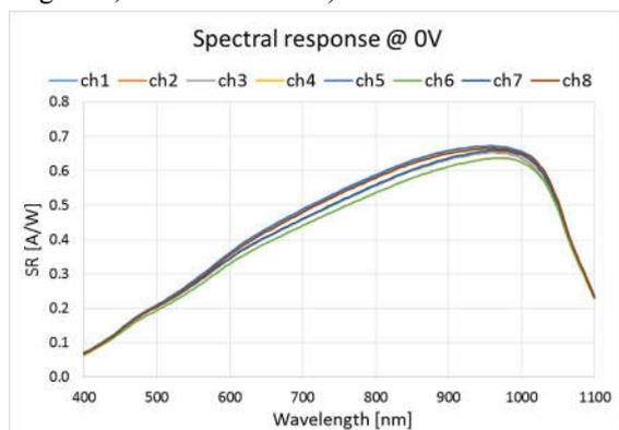
**Figure 2:** spectral response on a reference device
