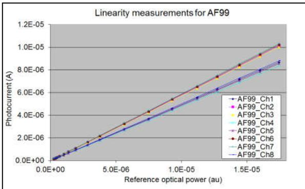
Figure 5: linearity measurement (power response)
