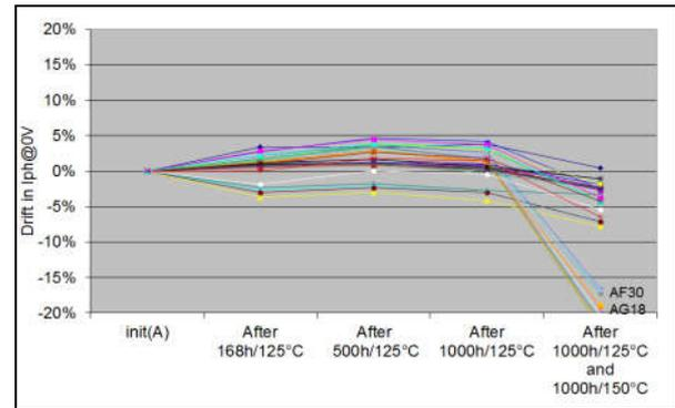
Figure 6: degradation of photocurrent on the second step of lifetest
