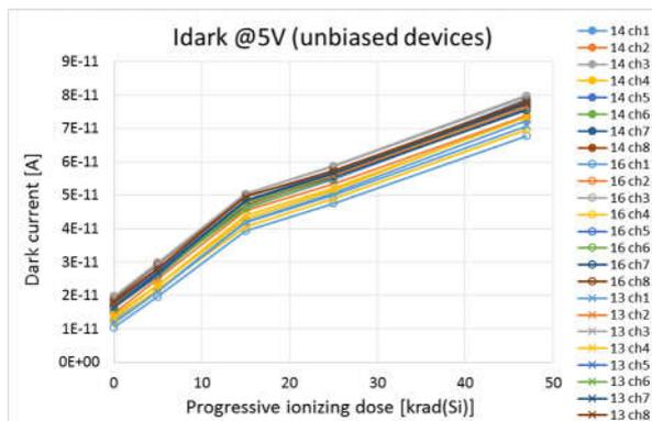
**Figure 7:** dark current degradation as a function of progressive ionizing dose, on devices unbiased during radiation
